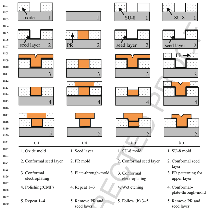
Fig. 3.21 Fabrication process comparison for one via and one upper conducting layer configuration: (a) damascene process; (b) conventional plate-through-mold process; (c) conformal plating process with etch back; (d) conformal plating without etch back [84] (Reprinted with permission. Copyright 2005 IOP)
